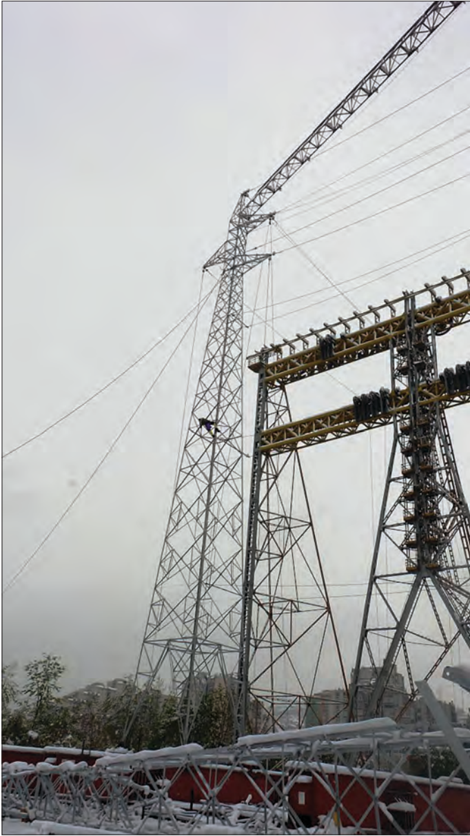
Figure 3.19 Energoinvest's test station for transmission poles, Alipašin Most a) Preparation for the test (left), b) Testing the bearing capacity of the power line pole (right)
