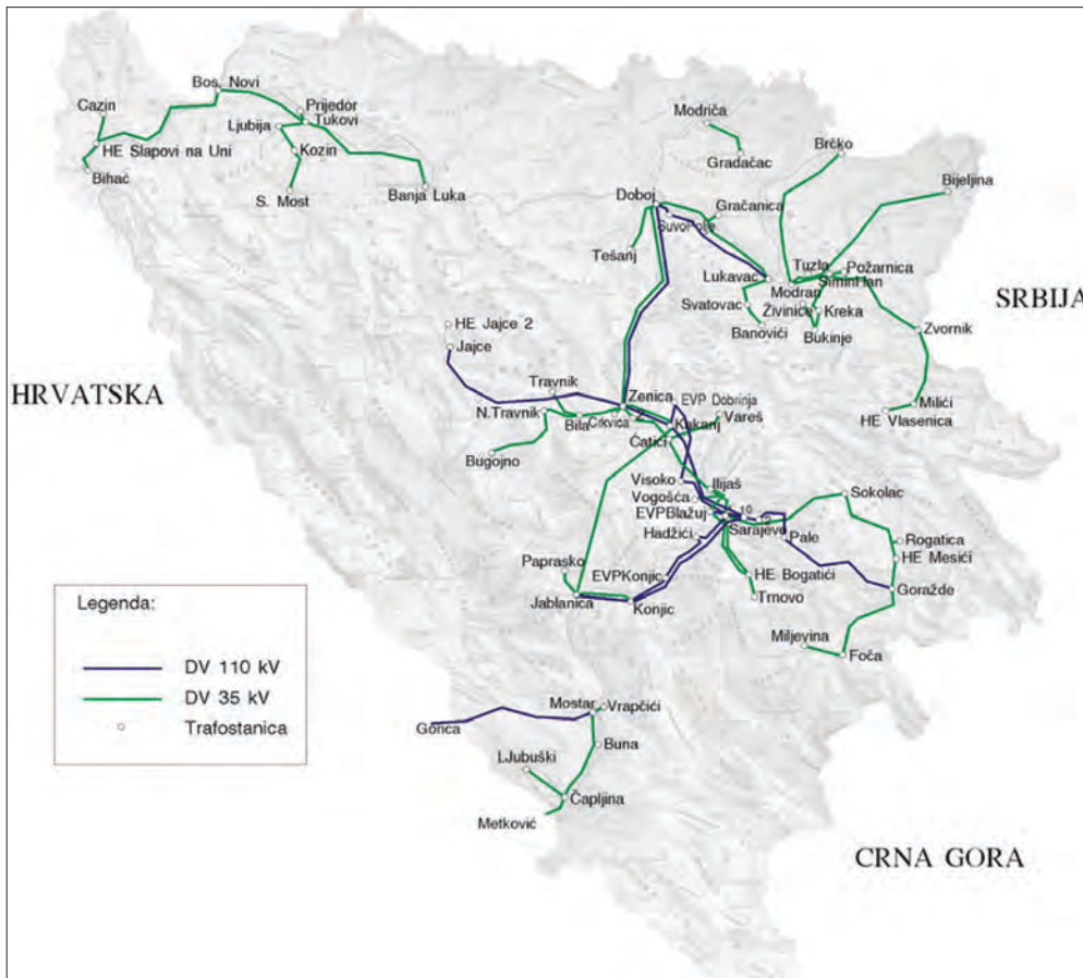
Figure 2.16 110 kV and 35 kV transmission network built by 1954
